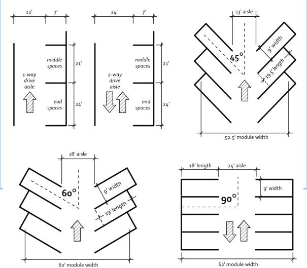
Note: Angled parking with two-way traffic shall be required to have an aisle width of no less than 24 feet.
