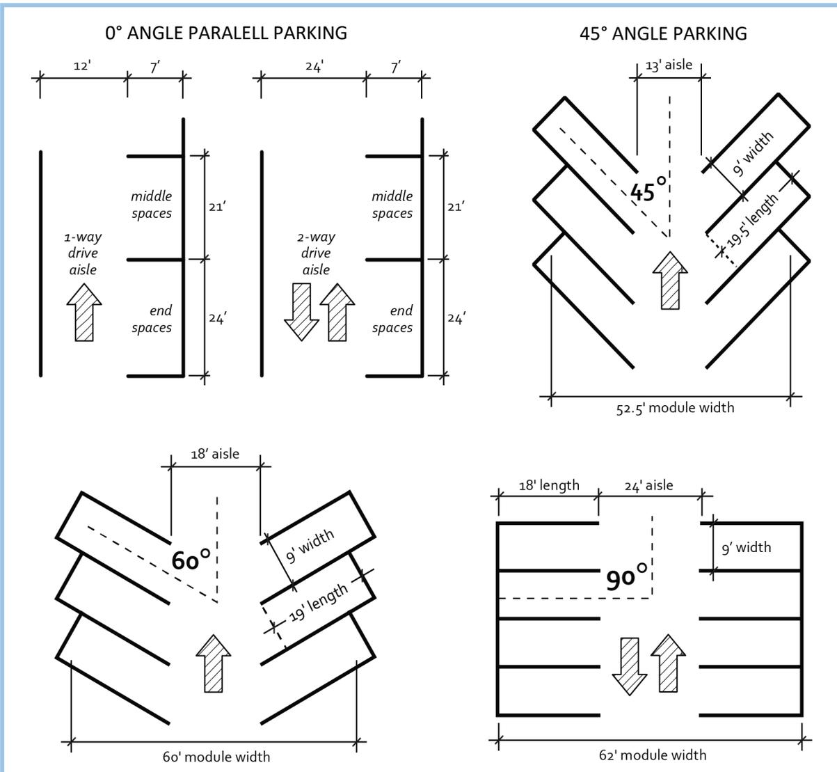
**Note: Angled parking with two-way traffic shall be required to have an aisle width of no less than 24 feet.**
